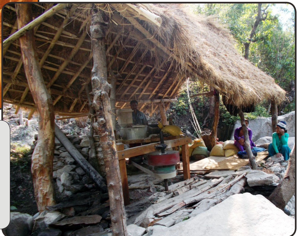
Right - A multi-purpose mill completed, servicing 6 villages (4 of HPC's villages and 2 from outside) and 60 households. The mill performs flour milling and rice de-husking, and can fit further attachments for vegetable oil extraction and planking.
