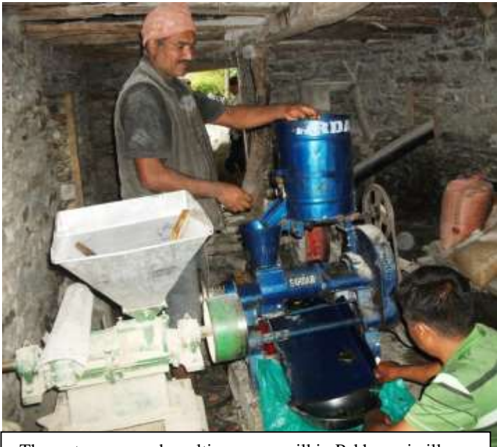
The water-powered, multi-purpose mill in Pakhapani village, here using the oil expelling part of the machinery, under the auspices of group member Om Bahadur Olli. The mill also grinds corn and wheat flour, and hulls rice. The mill services 9 villages in (4 of HPC's villages and 5 from outside) comprising 436 households (1550 men & women) .
